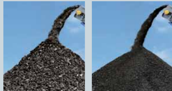
Final grain with high market value: grain size can be adjusted by regulating crushing speed to guarantee the highest quality.
