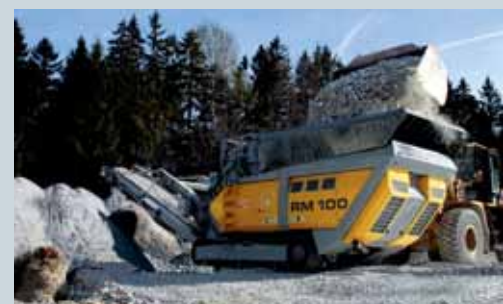
275 short tons homogenous 0/2.75" final grain: the RM100 delivers proven primary crushing performance in gravel pits.
